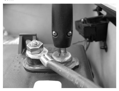
Figure 2: Probe is properly connected to the lead post
