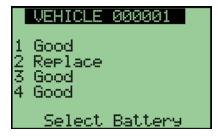
19. Use the arrow keys to select a battery and press **Enter**. The individual battery results are shown.
