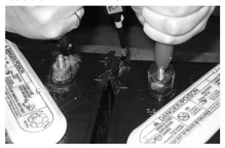
Figure 7: An Incorrect Way to Connect Probes
