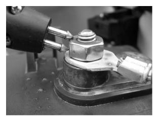
Figure 3: Probe incorrectly connected to the lead post
