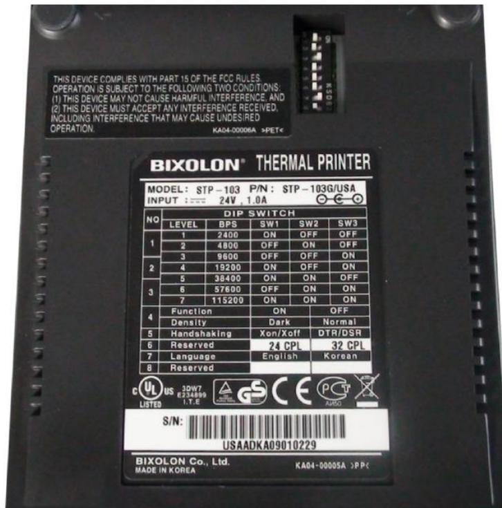
**Figure 1 - Bottom of Bixelon Printer**
