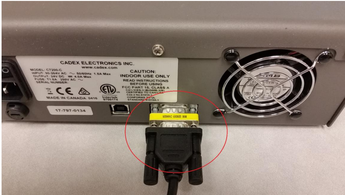
Figure 2 – C7x00/C7x00-C Back Connection
