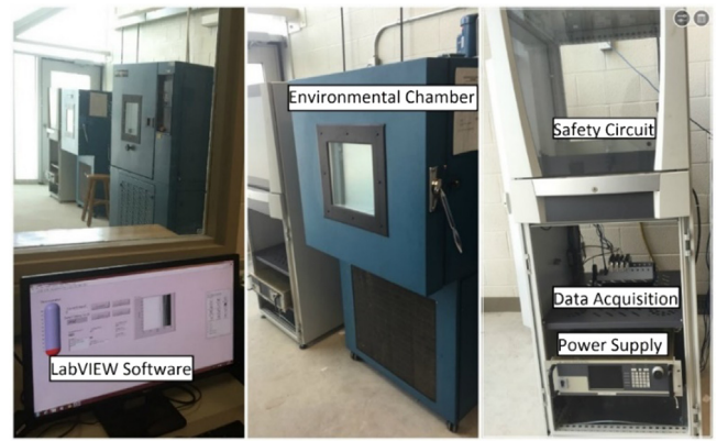
Fig. 3. Main components of the battery test setup located at CMHT.
