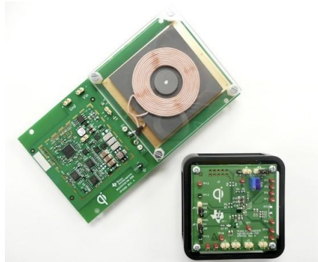
Figure 3: Wireless charging system by Texas Instrument
