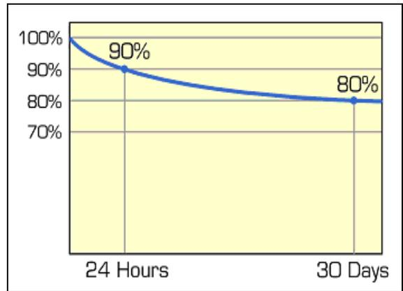
Lithium-ion has one of the lowest self-discharge. It loses less than five percent in the first 24 hours, and one to two percent thereafter. The mandatory circuit protection increases the discharge by another three percent per month. The self-discharge of all battery chemistries increases with rising temperatures, cycle count and advancing age.
