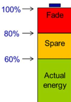
**Figure 2: Calculating spare battery capacity**
