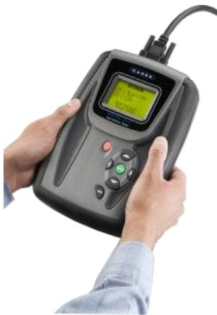
**Figure 3: Spectro CA-12 battery tester**
