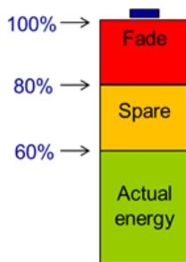
**Figure 1: Calculating spare battery capacity**
